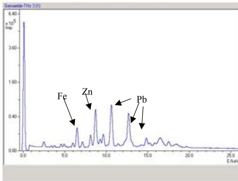
**Figure 2** X-ray spectrum of a single point measurement at the center of the woman's left eye on the painting sample
